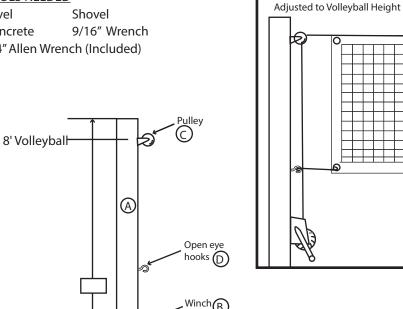
Slide all attachment hardware into the channel and secure at desired height.
